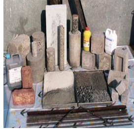
Concrete cored and sampled specimens
