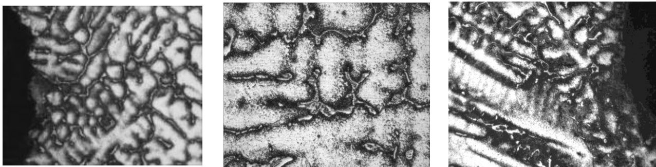
Figure 9 Alloy: ASTM A297 HP, Service exposed 29 years, 100mm away from rupture (in line of rupture), 100X, microstructures from OD (left), core and ID (right) show primary carbides at dendritic grain boundaries. OD and ID show intense tertiary creep cracking. Creep fissures are observed along primary carbide chain towards core. The secondary carbides area nearly absent within the grains. Sound attenuation measured is 56 to 58 dB
