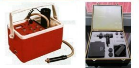
In-situ Metallography by replication method.
