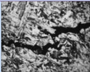
Corrosion fatigue SS 410 400X
