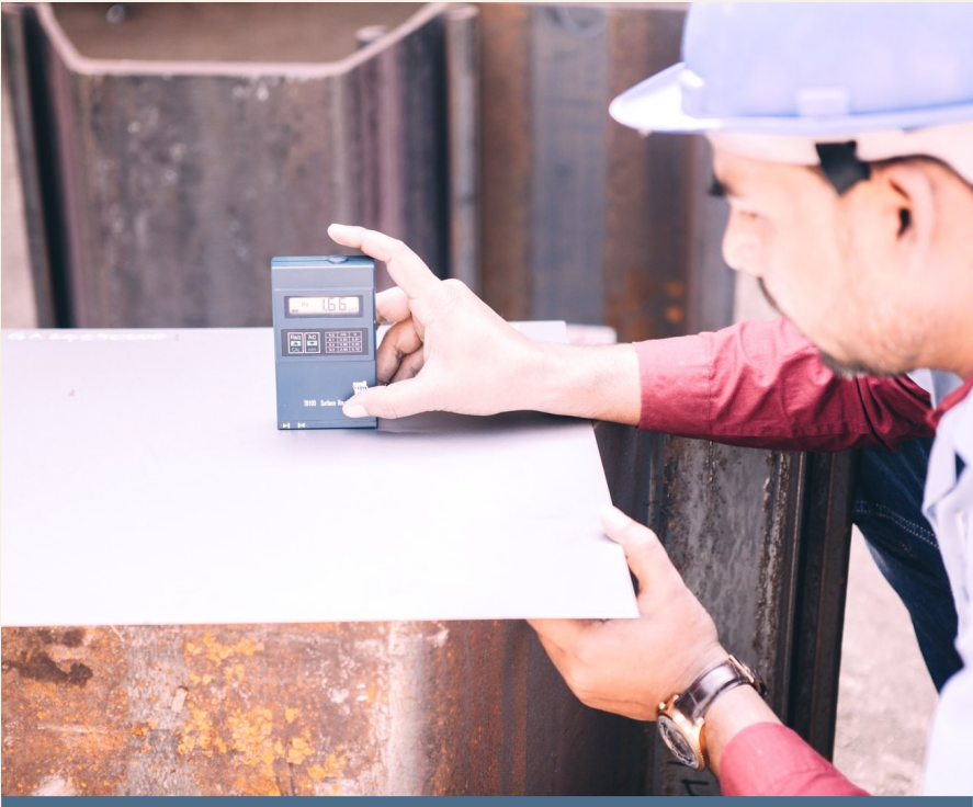
Ultrasonic thickness gauging on coated steel plate
