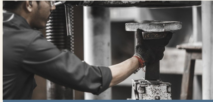
Concrete cube compression test
