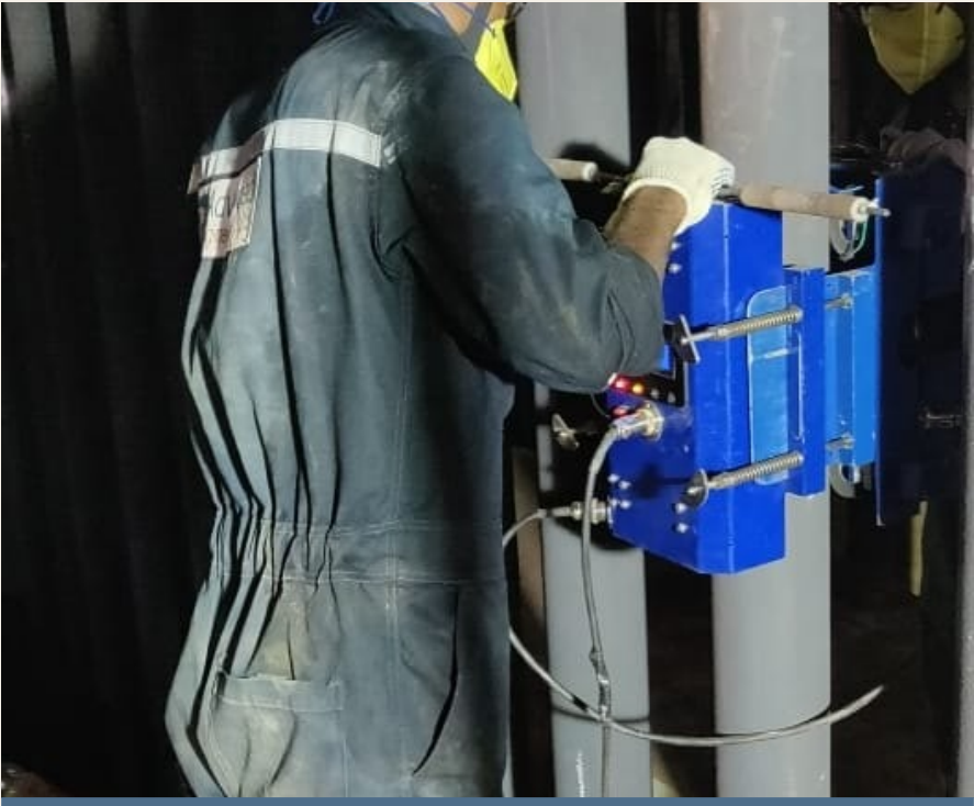
Robotic crawler being clamped onto a tube, TCR field team
