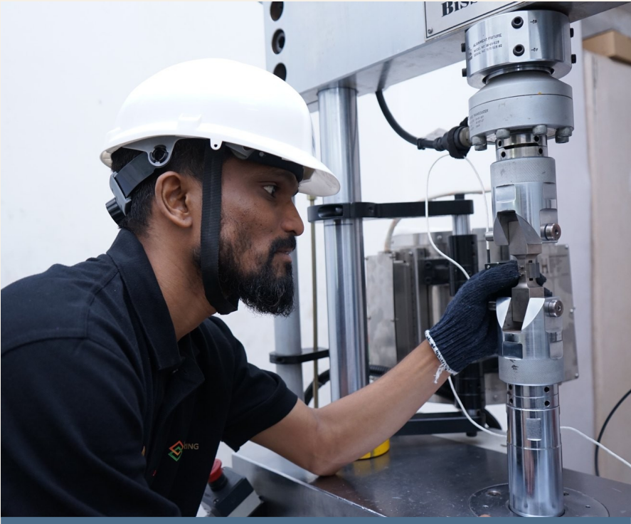
Specimen loaded in the grips of a servo-hydraulic test frame
