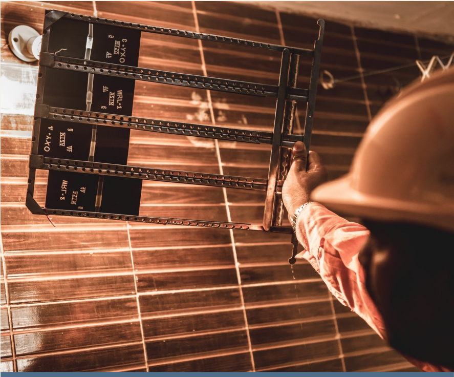
Weld radiographs coming out of the processing tank
