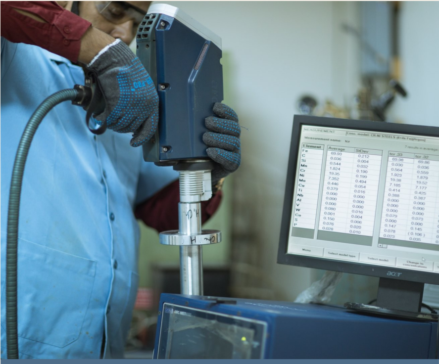
Alloy identification, the result read on screen
