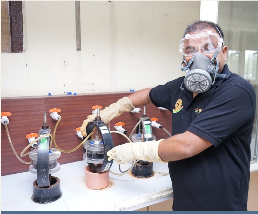
Sulphide stress cracking proof rings in sour test cells
