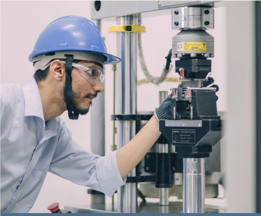
Tensile specimen set in the 50 kN universal testing machine
