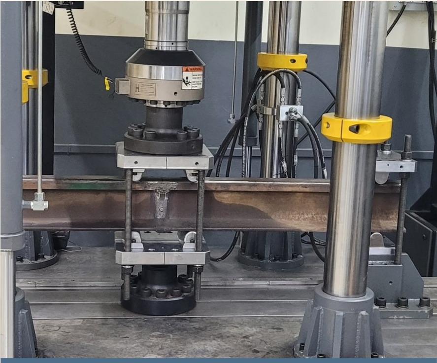
Rail section set up for fatigue testing
