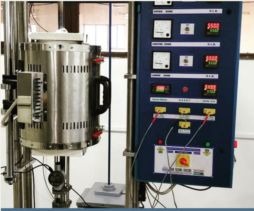
Creep frame with three-zone furnace and controller
