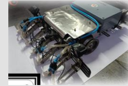
Tank Shell UT Scanning_ Vertical Movement
