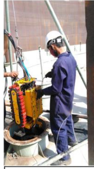
Thru 24" Dia Manhole -Single Deck Floating Roof Tank
